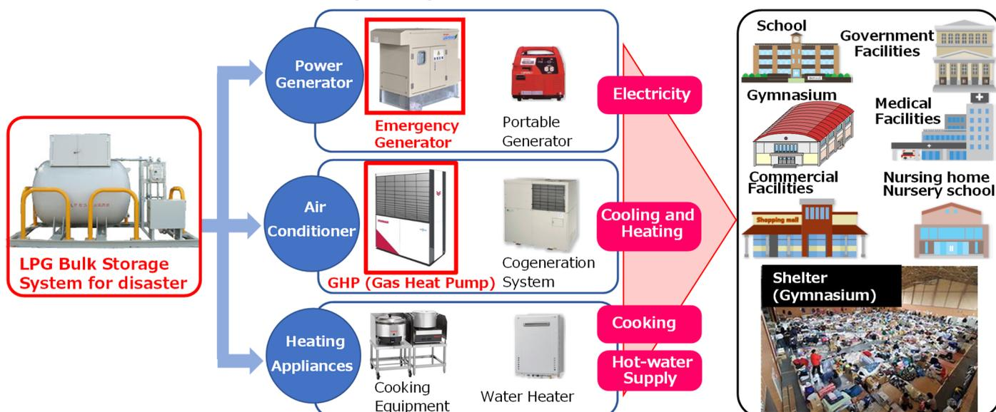
Figure 6: Disaster response of LPG disaster bulk system (Source: JLPGA)
