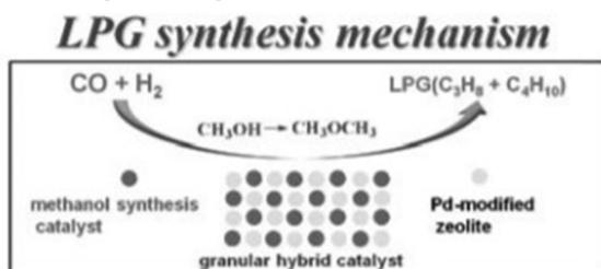
**Figure 3: The scheme for LPG synthesis**
