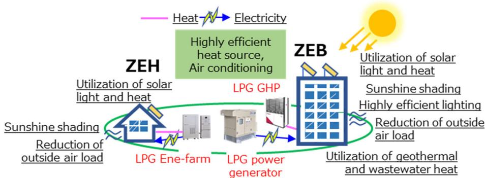
Figure 8: Conceptual diagram of ZEH/ZEB (Source: JLPGA)
