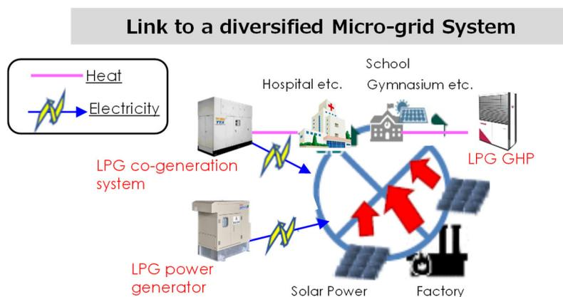
**Figure 5: Conceptual scheme of Decentralized Micro-grid System where LPG could contribute**
